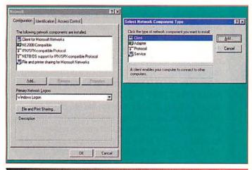
FIGURE 4 Using the Network Control Panel, you can add the four types of network components (right). When you're done, your configuration should look something like the left panel.
