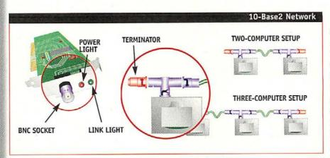
FIGURE 2 Using RG-58 cable and BNC connectors (also known as 10-Base2), you can daisy-chain multiple rigs together to form your own network. The last machine in the chain needs to have a terminator (inset).
