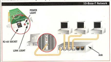
FIGURE 3 A 10-Base-T network is another option, if you want to have a hub. This doesn't require daisy-chaining, so you won't need to fuss with T-connectors, but the hub itself will run between \$90-\$150. Inset shows RJ-45 connection into a network interface card (NIC). The two lights indicate power to unit and that a connection has in fact been made with another system.
