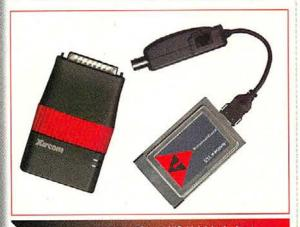
LAPTOP CONNECTORS The PC card NIC (right) is the least expensive means of connecting a laptop to a network. It plugs into a PC card slot and accepts an RJ-45 or a BNC connection; the Linksys PC card shown accepts both connectors. If your laptop doesn't have a PC card slot, the parallel port ethernet adapter (left) is the alternative, but it's much more expensive. The adapter plugs into the parallel port and accepts an RJ-45 (10-BaseT) connection.
